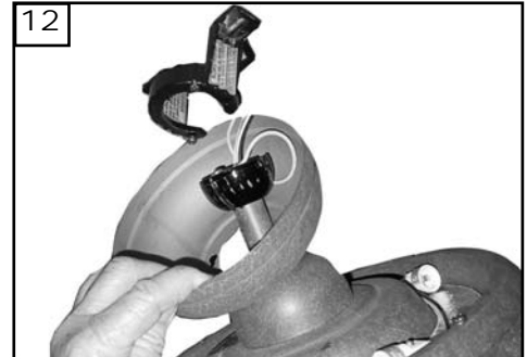
12 Raise fan with downrod assembled to the ceiling bracket and hang fan assembly. Be sure to rotate the downrod ball so that the notch in the bracket engages the slot in the ball.
